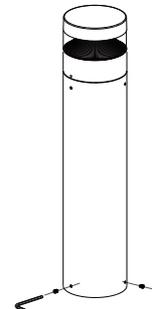
Secure the body to the base plate with the HEX screws, turn on mains supply and test for correct operation
